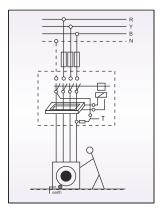
The RCCBworks on the current balance principle.the supply conductors,i.e.,the phases and the neutral,are passed through a torroid and from the primary windings of a current transformer.lts secondary winding is connected to a highly sensitive electromagnetic trip relay,which operates the trip mechanism.
